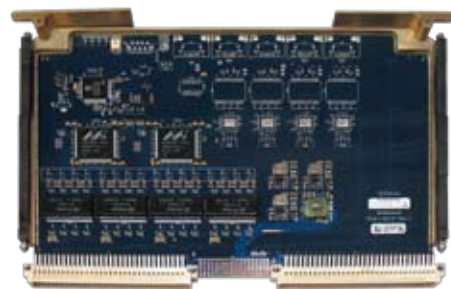
VME Ethernet Switch
